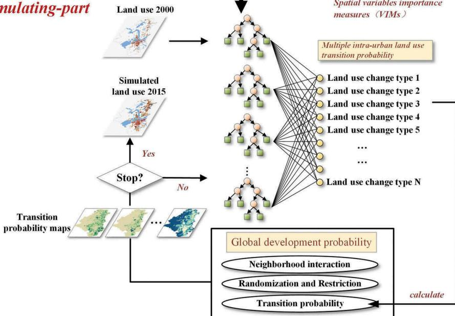
Figure 1. Structure of the RF-CA model.
