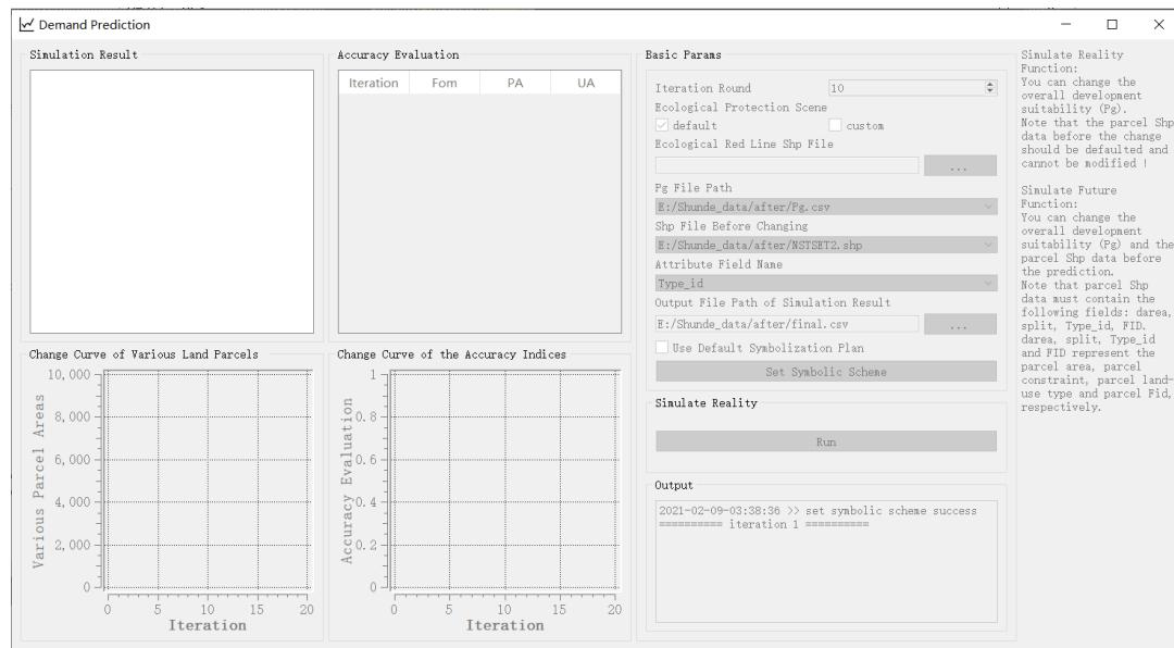
The system will display the land-use simulation map generated by the last iteration round in tandem with the accuracy evaluation indexes with each iteration at the top left corner of the panel. At the bottom left corner, the system will display the diagram that records the land-parcel area change with each iteration, as well as the simulation accuracy change with each iteration, respectively.
