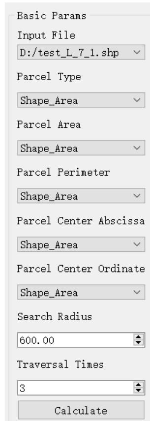
Search radius, the sixth parameter, sets the initial radius value for optimal search radius mining. The parameter has to be manually *entered* by users.
