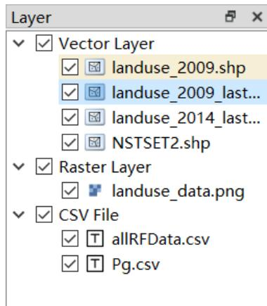
To determine a specific GIS operation, **Right-Click** the selected data and a GIS operation widget will pop up on hand. Available GIS operations include “Zoom to Layer”, “Show Attribute Table”, “Select the Current Layer to Operate”, “Edit Vector Symbol”, and “Remove Layer”.
