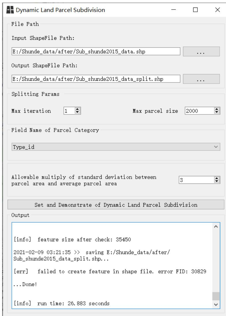
Users can **re-select** files and **re-set** parameters for the next round of DLPS demonstration. The parameters from previously completed demonstrations would be automatically uploaded to the system for subsequent processing. A LOG output interface is provided to check the output info, which is shown as below:
