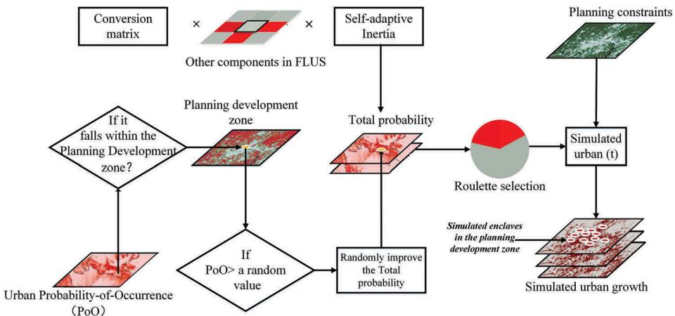
**Figure 3.** Flowchart of the random seeding mechanism for considering the influence on the planning development zone.
