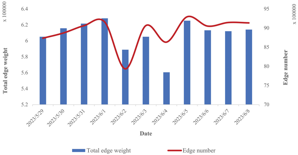
Figure 4. Temporal changes in the total edge weights and the edge numbers of the network within the observation window. Here, the total edge weights represent the total origin–destination flux, and the edge numbers represent the degree of connectivity between the grids.
