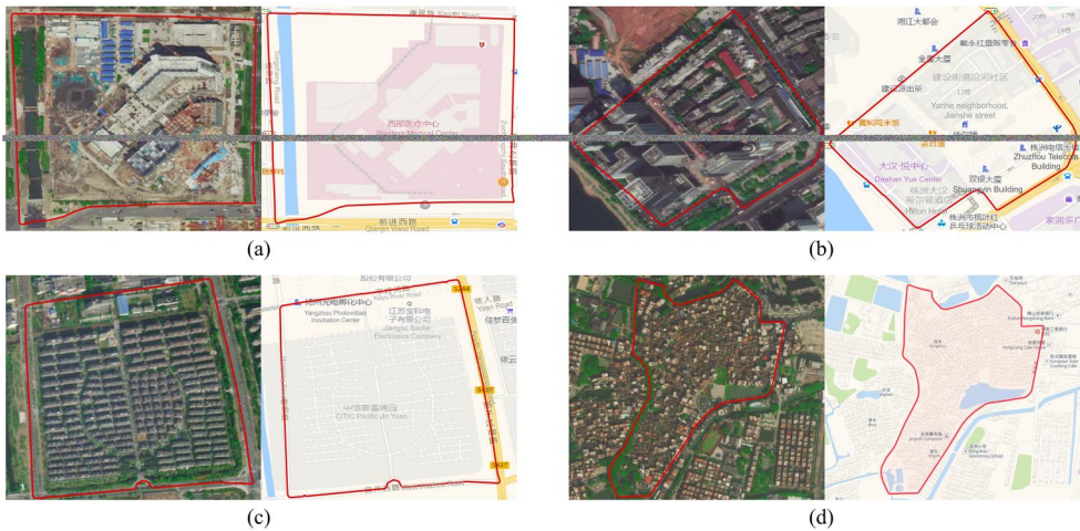
Figure 8. Typical examples of labeling errors. Errors that occur due to the misleading of pre-labeling include (a) industrial land being labeled as public services land and (b) mixed land-use being labeled as commercial zones. Errors that occur due to the confusion in second-level land-use categories include (c) ‘villas and high-end residences’ or ‘high-rise residential buildings’ and (d) ‘urban village’ or ‘rural homestead’.
