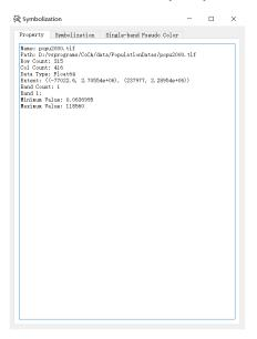
The "Properties" page displays the basic parameters of the selected layer, including the layer name, path, resolution, data storage type, extent, number of bands, and the maximum and minimum pixel values for each band.
